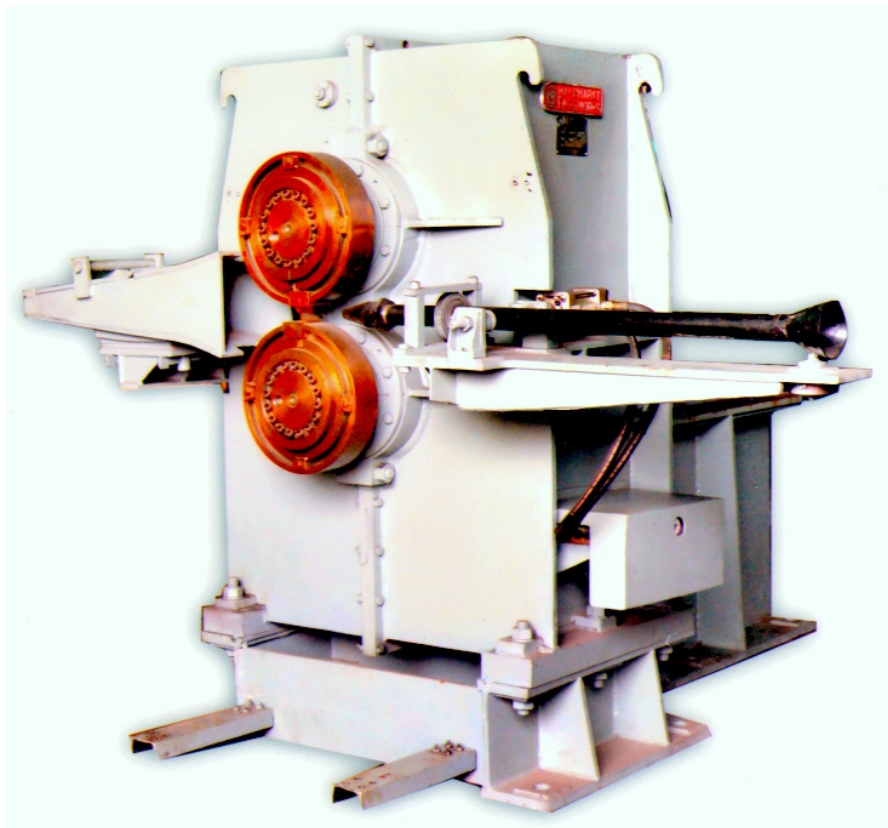
High Speed Continuous Rotating Shear to cut 8mm at 24m/s, 12mm at 14m/s
